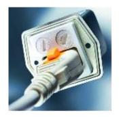
The compact module combines an appliance inlet, fuseholder, and standard or medical EMC filter rated up to 8 A at 250 VAC. The original 5707 offers IP 65 seal protection at the panel opening, around the fuseholders, and between the inlet and connector pins. The module can also be fitted with an additional gasket in the inlet cavity for IP 54 protection between the inlet and the cord connector. A V-Lock cord set prevents unintentional disconnection.
