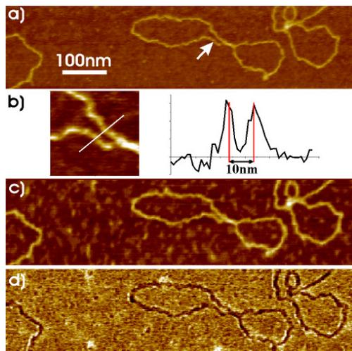
Images taken on a 6 day old sample in the area of a single graphene: (a) Topography image recorded in contact mode under a normal force of 25 nN. Arrow indicates an area enlarged on (b) with two resolved DNA strands running nearly parallel to each other at a distance of 10 nm, as visualized by the inserted cross section. (c) Intermittent contact mode topography image acquired a few minutes after (a) with the same tip. (d) Intermittent contact mode phase contrast image of the same area.\*
