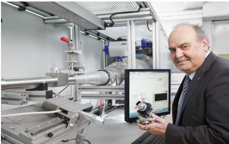
Before going into series production, the EGR valves undergo extensive tests including endurance. Osman Sari, Pierburg's chief developer of the new compact EGR valve at a flow test rig.
