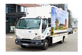
The drive system is based on the HyRange® fuel cell system combined with a battery. This system meets demands in respect of range, payload and costs, with zero emissions and low-noise drive.
