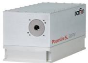
PowerLine SL PV series provides for excellent longterm stability in regard to high performance: selfactuating thermal monitoring, stabilization of all relevant optical components with Peltier elements and heat dissipation with an air- or water-cooled cooling plate.
