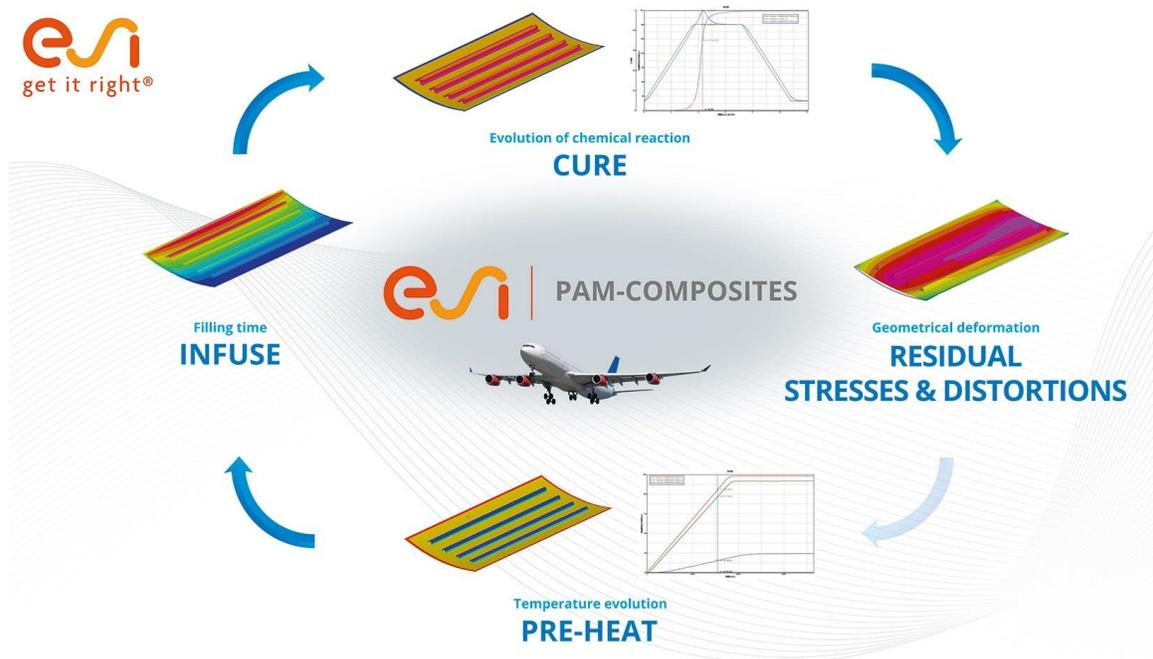
Image: Sample application: PAM-COMPOSITES can predict the entire manufacturing chain for developing a defect-free aeronautic composite fuselage panel.
