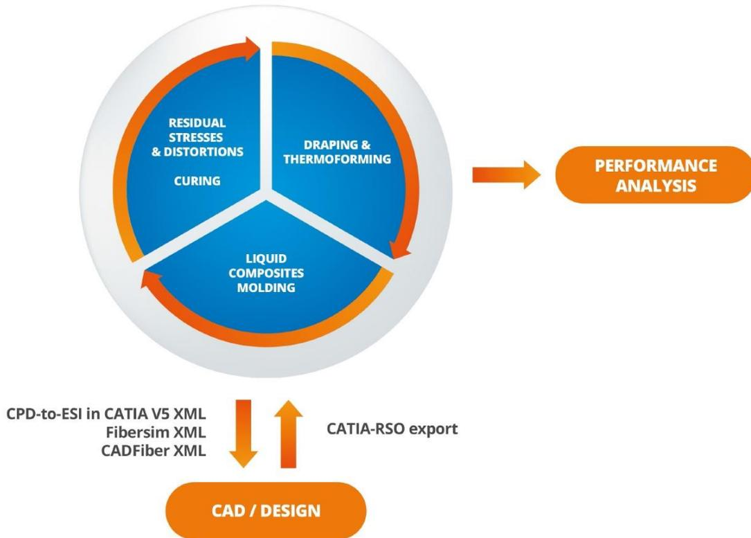
Image: ESI PAM-COMPOSITES enables the prediction, analysis and correction of manufacturing defects for composite structural components across the complete manufacturing chain. Manufacturing processes covered include draping, thermoforming, Liquid Composites Molding (LCM), Resin Transfer Molding (RTM), and curing.
