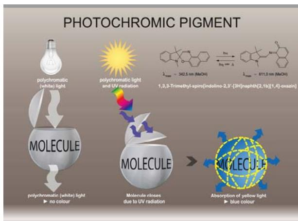
When working with photochromic pigments, Hohenstein researchers take advantage of the effects of the subtractive colour mixture: UV radiation causes the molecular bonds in photochromic pigments to change. The yellow portions are subsequently filtered out of the incident white light, so that observers now perceive the formerly invisible/colourless pigment as blue.
