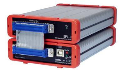
The 5V auxiliary voltage, led out at pin 17 of the 37-pole Sub-D socket of the logger, supplies the *BP16* with power and turns it on and off.
