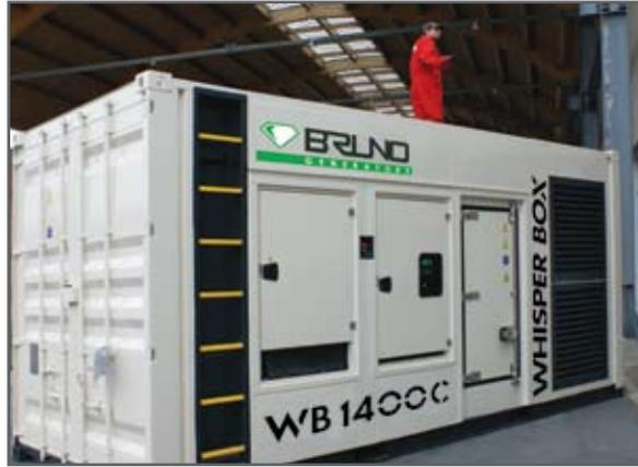
◀ **3** Side ladder. Easy access to the roof for visual inspection, maintenance, radiator refueling
