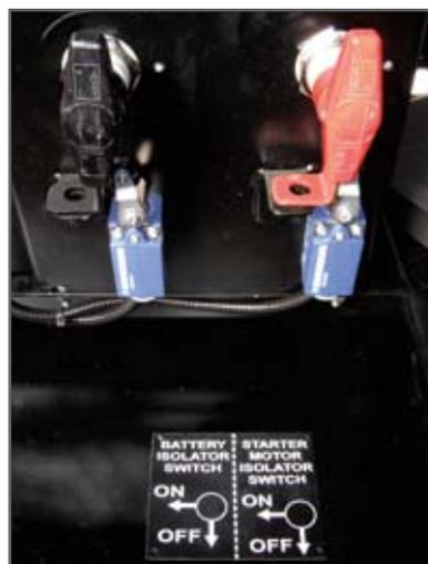
◀ Lockable disconnectors for starter motor and battery (mining applications)
