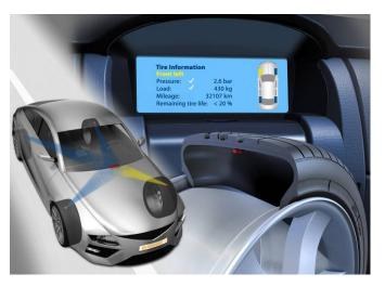
Intelligent tire sensors, which are integrated into the tires, deliver information about the current tire distortion of the rolling tire.
