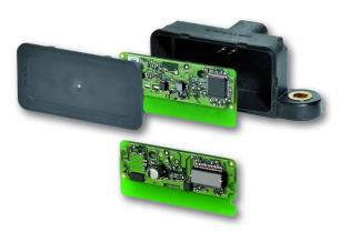
The sensor cluster provides all control units in the vehicle with the vehicle's current movement status (yaw rate, longitudinal and lateral acceleration and, optionally, pitch and roll rates).
